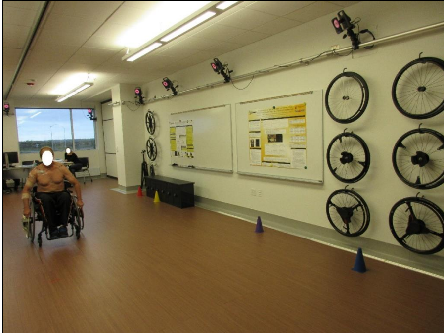
Figure 11. A subject propelling on a tiled level floor using the IntelliWheels geared manual wheelchair wheels.
