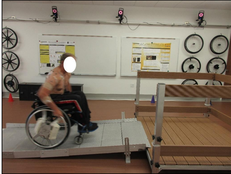
Figure 12. A subject ascending a ramp using the IntelliWheels geared manual wheelchair wheels.
