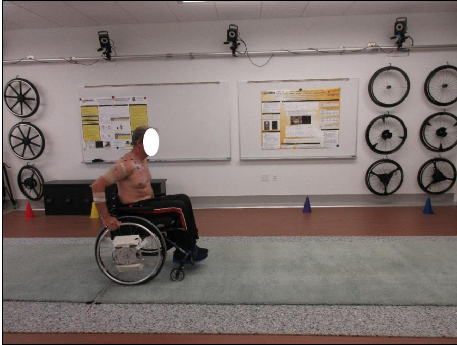
Figure 10. A subject propelling on a carpeted level floor using the IntelliWheels geared manual wheelchair wheels.
