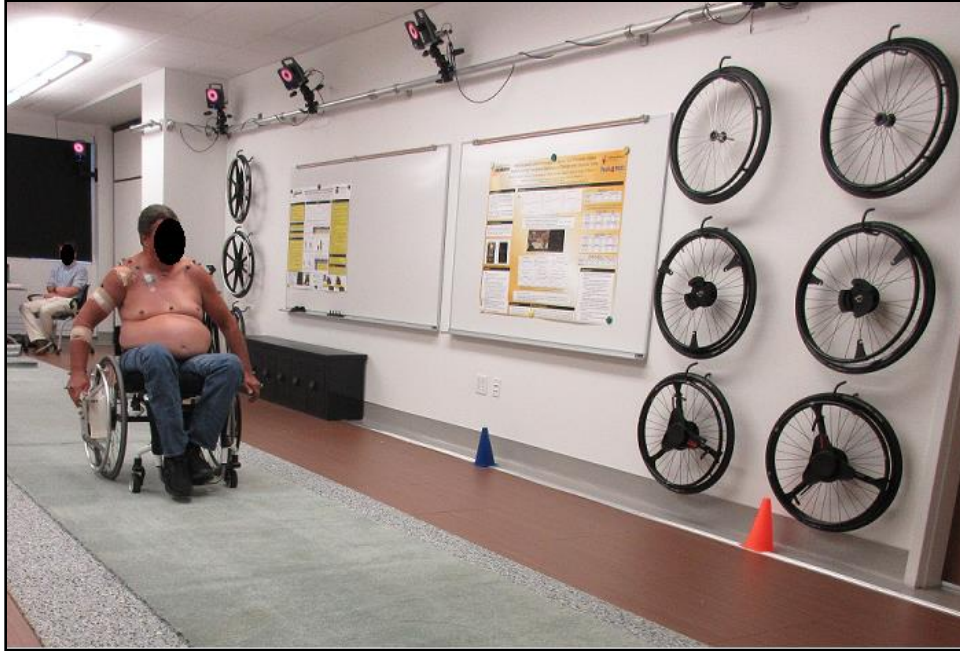
Figure 30. A subject propelling on a carpeted level floor using the IntelliWheels geared manual wheelchair wheels.
