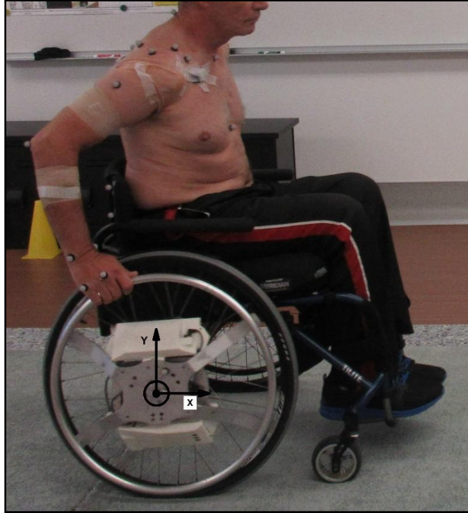
Figure 31. A subject propelling the instrumented geared wheel on a carpeted level floor. The instrumented hand-rim global coordinate system follows the right-hand rule with the positive X -axis anterior, positive Y -axis superior, and positive Z -axis pointing out of the wheel along the axle. The picture also depicts the subject instrumented with the motion capture markers and surface electromyography electrodes.
