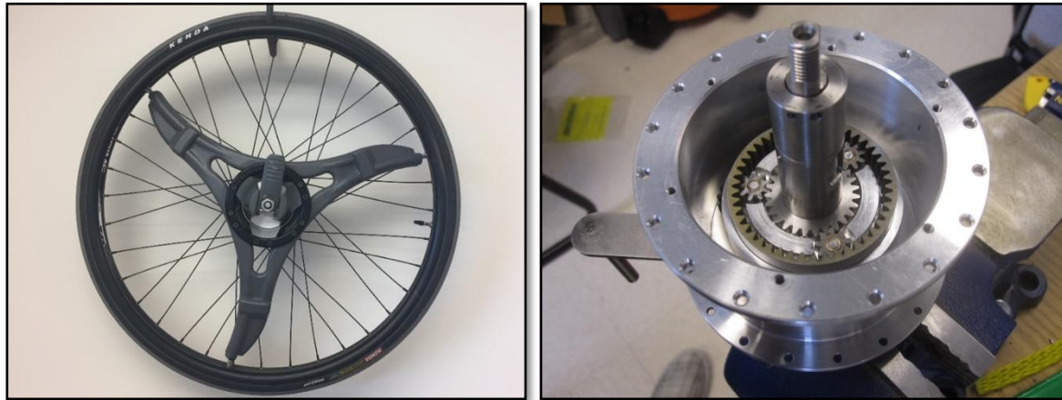
Figure 8. IntelliWheels geared manual wheelchair wheel (left) and the planetary gear train from a prototype IntelliWheels geared manual wheelchair wheel (right).
